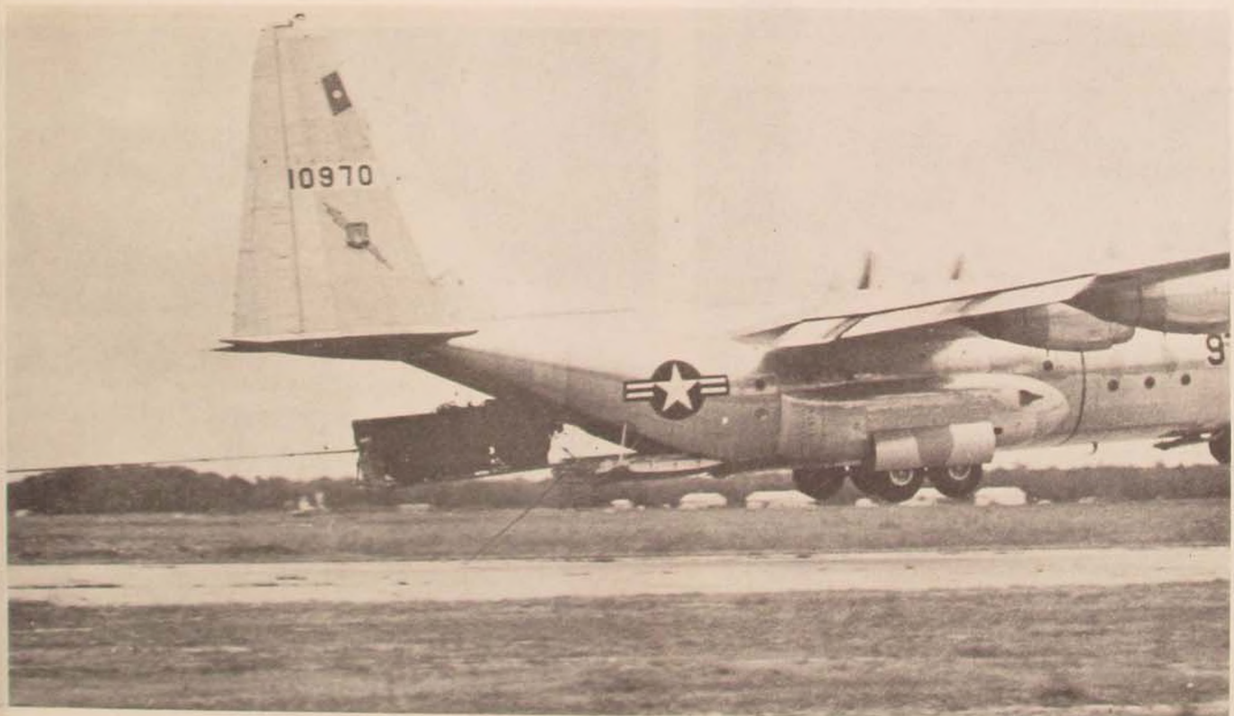
Making a pass over the drop zone at approximately five-foot altitude, a C-130 deploys a parachute that unloads a 3-ton truck by the ground proximity extraction system (GPES).
