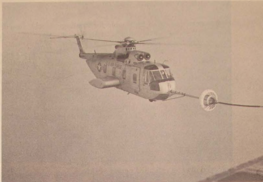
First hookup of CH-3C with KC-130F tanker proves feasibility of aerial refueling technique.
