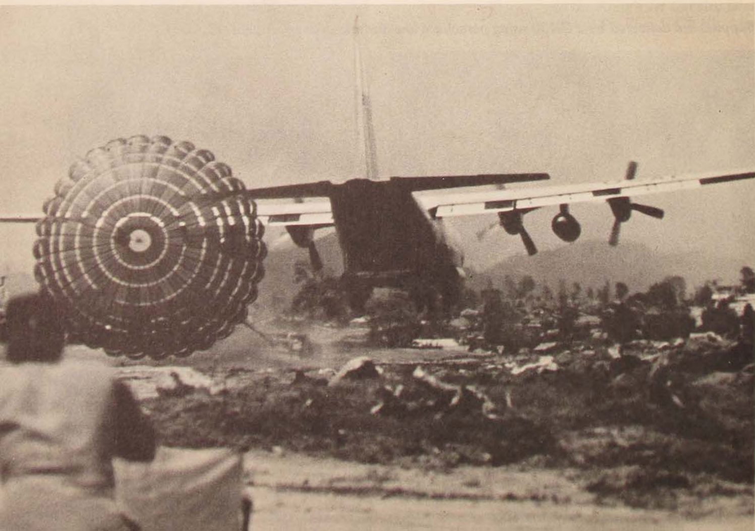
With LAPES (low-altitude parachute extraction system), platform-mounted loads are pulled from a C-130 transport at about five-foot altitude. The system is used for resupply to narrow drop zones.
